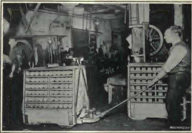
Fig. 3. Truck built by the Chapman Double Ball Bearing Co. for transferring Shrapnel Shells about the Shop
